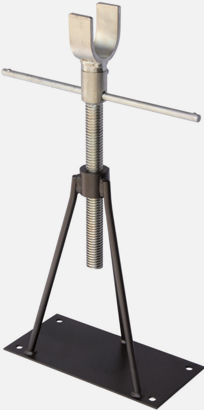
Mechanical Reel Lifting Support The Arvi Mechanical Reel Lifting Support, used in pairs, hold coils made of various materials, including electrical and telecommunications. This mechanical version allows manual adjustment via a screw mechanism, ensuring safety and efficiency.
